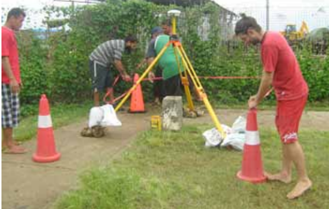
Setting up the Base Station for Real Time Kinematic survey.
