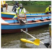
Caption: SOPAC and Water Authority of Fiji takes measurements in the Rewa River with a Current Flow Metre, a part of the Rewa Flood Forcasting
