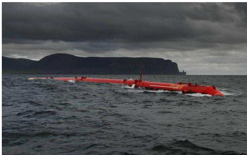
Figure 2.2 Pelamis device deployed in Scotland
