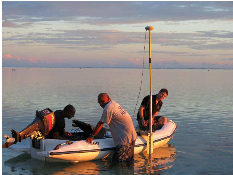
Figure 3.2 Boat setup for the lagoon/reef flat bathymetry survey
