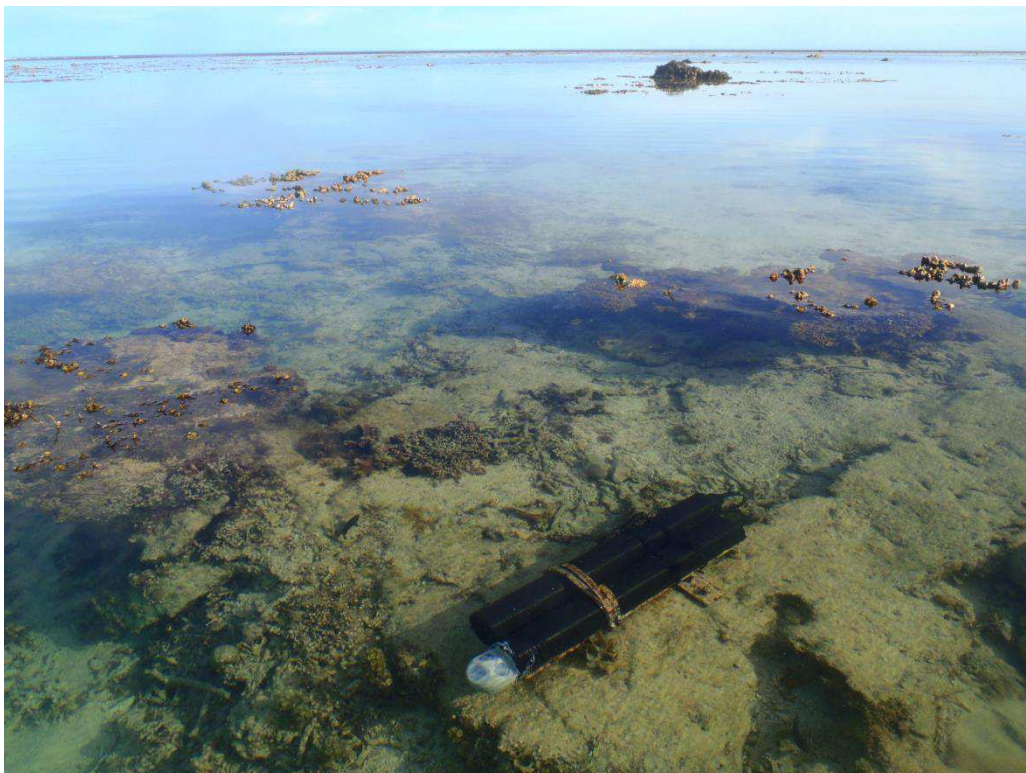
Figure 3.4 Aquadopp deployed near the centre of the reef flat in Maui Bay
