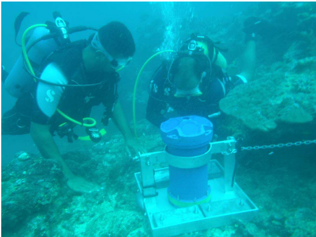
Figure 3.6 RDI-Workhorse (University of Auckland) deployed on the reef slope of Maui Bay in 20m depth
