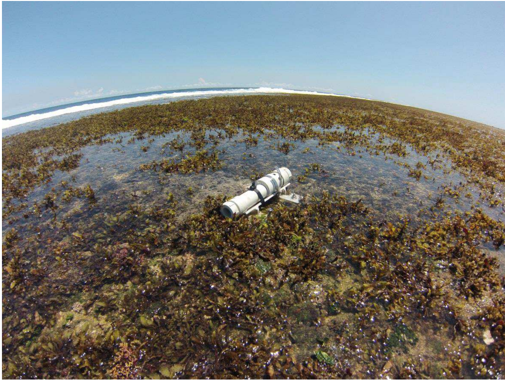
Figure 3.5 RBR-TWR deployed near the reef crest in Maui Bay
