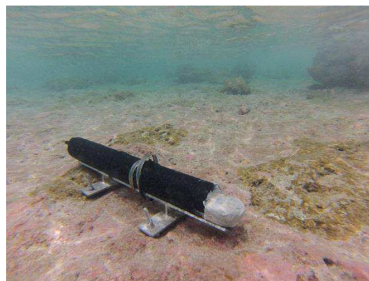
Figure 3.4 Aquadopp deployed near the centre of the reef flat in Fatato
