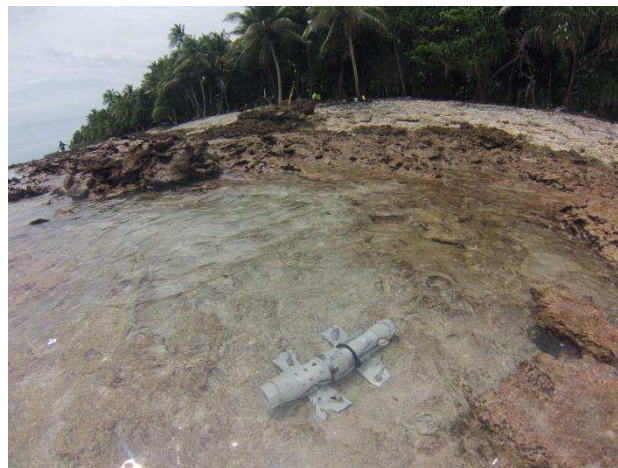
Figure 3.3 RBR-TWR deployed near the shore in Fatato
