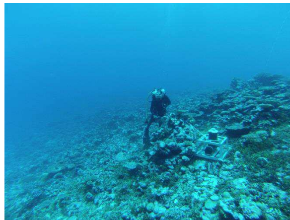
Figure 3.6 AWAC deployed on the reef slope of Fatato in 20m depth
