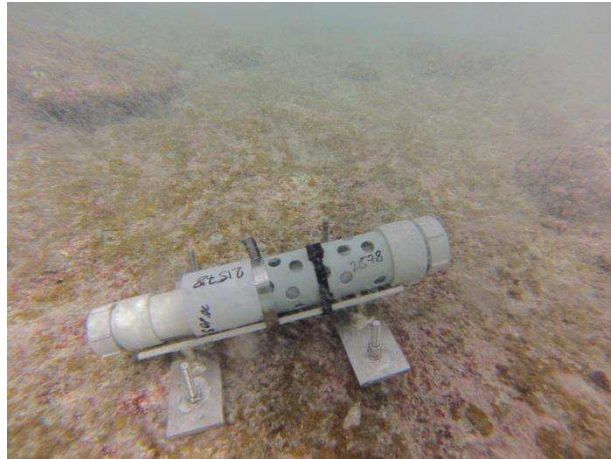
Figure 3.5 RBR-TWR deployed near the reef crest in Fatato
