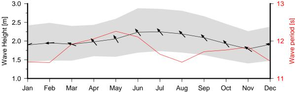
**Figure 4** Monthly wave height (Black line), wave period (Red line) and wave direction (arrows). The grey area represents the range of wave height between calm periods (10% of lowest wave height) and large wave events (10% of highest wave height)
