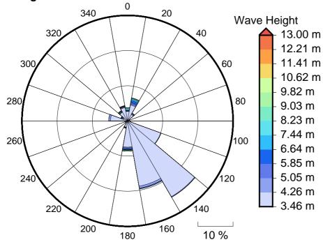
Figure 6 Large, severe and extreme wave roses for Fugro Directional Wave Buoy
