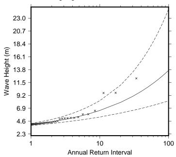
**Figure 9** Extreme wave distribution for Fugro Directional Wave Buoy. The crosses represents the wave events that occured since 1979. The plain line is the statistical distribution that best fit the past wave events. The dotted line show the upper and lower high confidence of the fit, there is a 95% chance that the fitted distribution lie between the two dashed lines.
