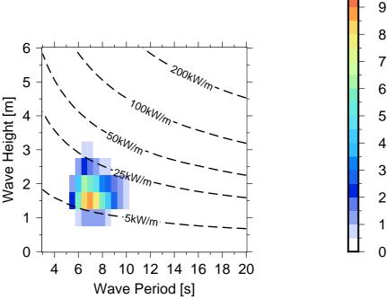
Figure 10 Occurences of sea states in Fugro Directional Wave Buoy .
