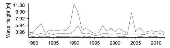
**Figure 8** Annual variation in large waves (90th percentile)(lower curve), severe waves (99th percentile) (middle curve) and the largest wave(upper curve) in Fugro Directional Wave Buoy.
