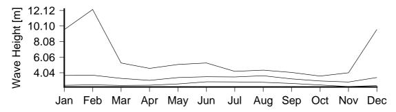
**Figure 7** Monthly variation in large waves (90th percentile)(lower curve), severe waves (99th percentile) (middle curve) and the largest wave(upper curve) in Fugro Directional Wave Buoy.
