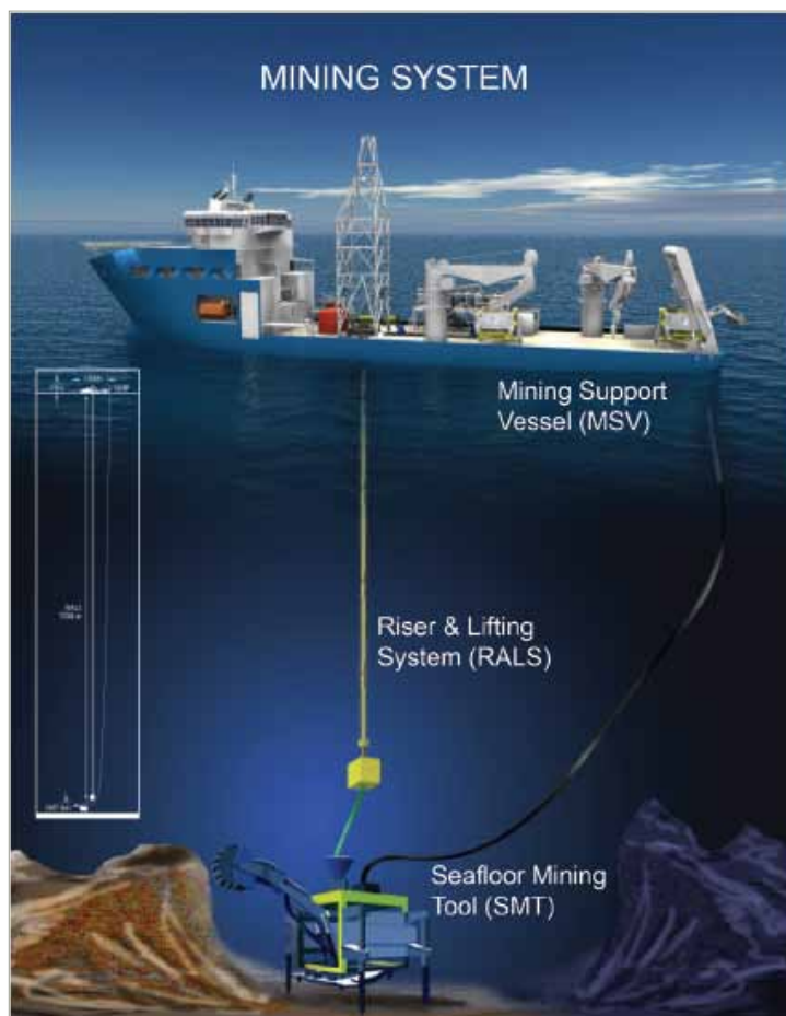
A configuration of the planned Nautilus Minerals Seafloor Mining System (Nautilus Minerals, 2009)
