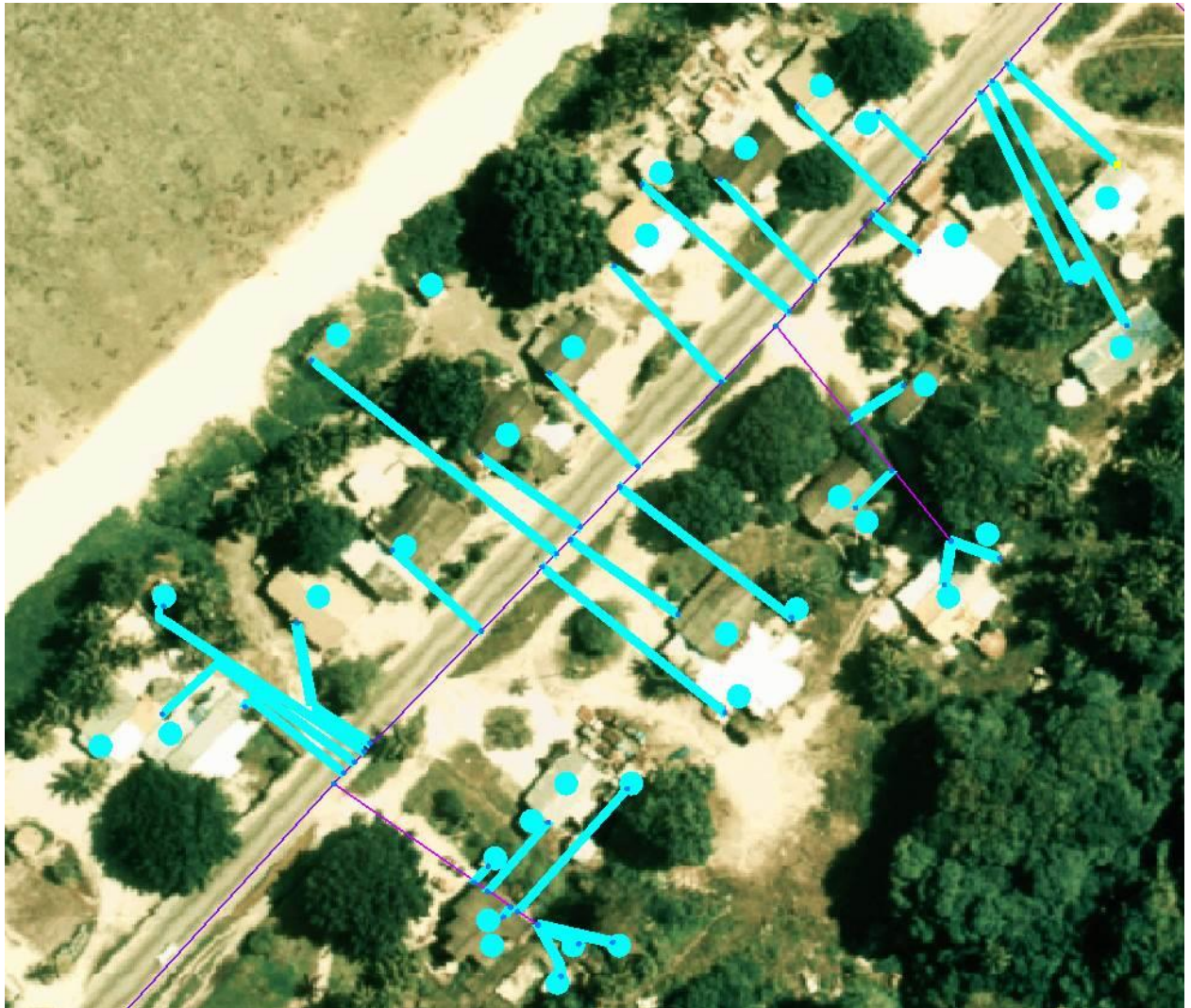
Figure 92. Sample customer connection pipework in northwest Nauru
