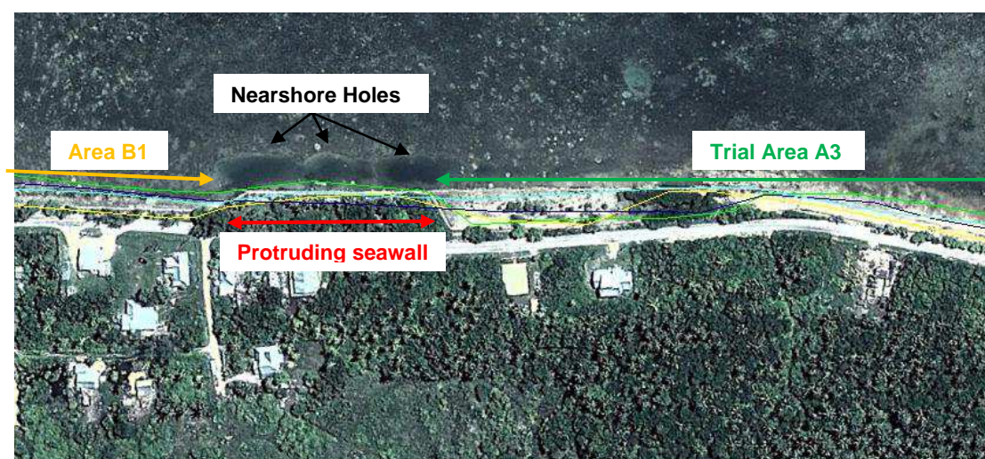
Figure 2.5. The Area A3 trial site is effectively separated from Area B1 to the west by the protruding seawall and nearshore holes.
