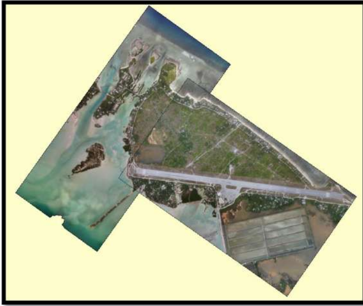
Figure 26. Combined orthophotos from flight 1 and flight 2; 10 cm image resolutions.
