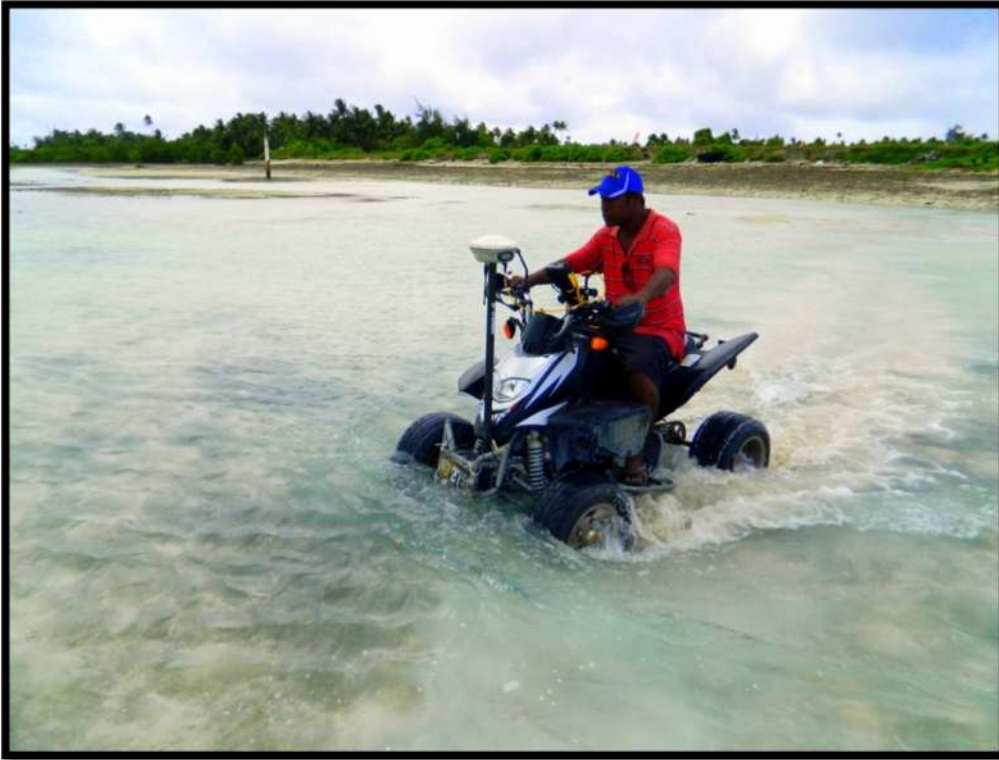
Figure 11. A Trimble R8 was mounted on a quad bike to help collect data from the sand flats as well as the water reserve.
