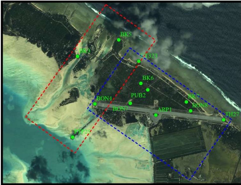
Figure 16. Coverage of the UAS survey; flight 1 covered an area of 2.4 km 2 (the red zone), and flight 2 covered an area of 2.6 km 2 (the blue zone).
