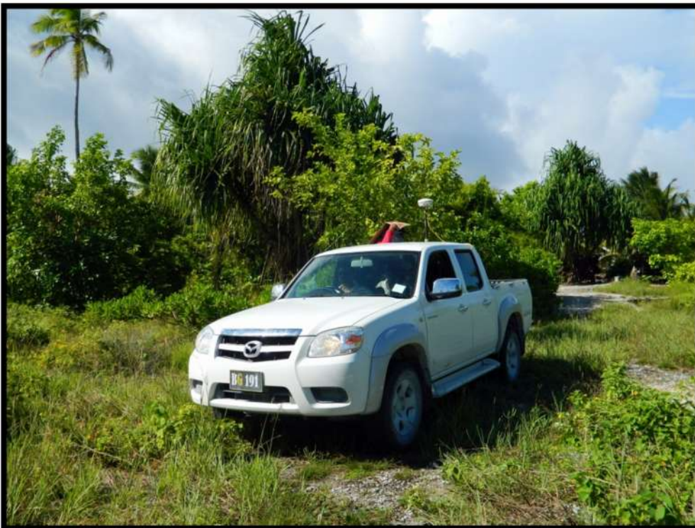
Figure 10. GPS receiver mounted on a government pick-up truck. The rover (receiver) and its pole are mounted at the back of the truck. The controller is mounted inside the car to allow a real-time check of data.
