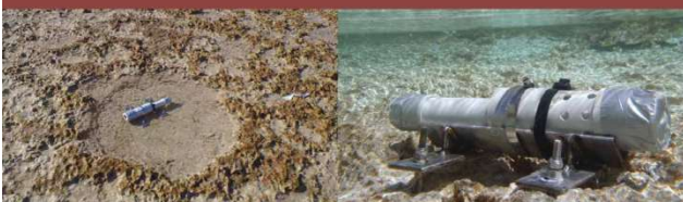
This Tide and Wave Recorder measures tides, temperature and waves.
