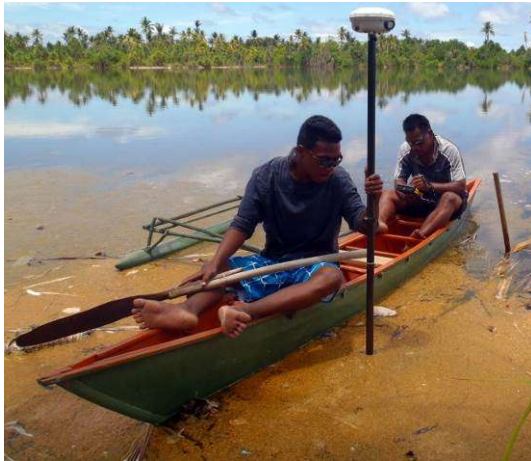
Figure 6. A canoe was used for an RTK survey in the lakes and saltwater marshes
