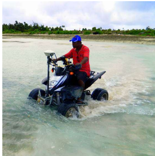
Figure 5. Trimble R8 was mounted on the quad bike to assist with RTK survey coverage on the sand flats as well as the water reserve
