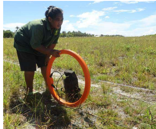
Figure 8. Water Engineering Unit (WEU) staff discussing resistivity survey methodology (left) and WEU staff undertaking EM34 survey work (right)
