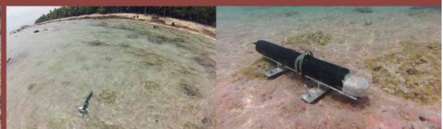
This Acoustic Doppler Current Profiler measures current speed & direction, temperature and pressure.
