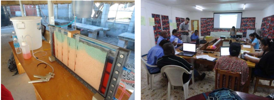
Figure 9. Physical model of atoll hydrogeology used for demonstration during workshop (left). Workshop attendees developing simple groundwater model (right)
