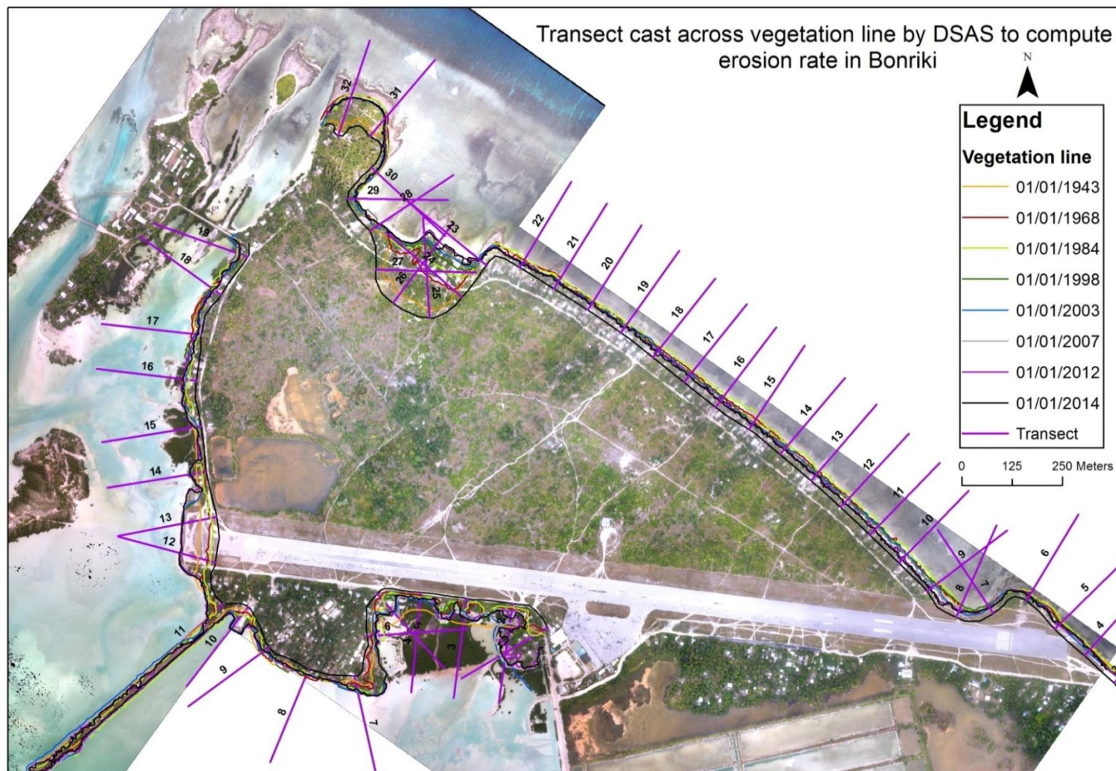
Figure 4: Transect cast used for Digital Shoreline Analysis System analysis for vegetation line from 1943 to 2014 at Bonriki
