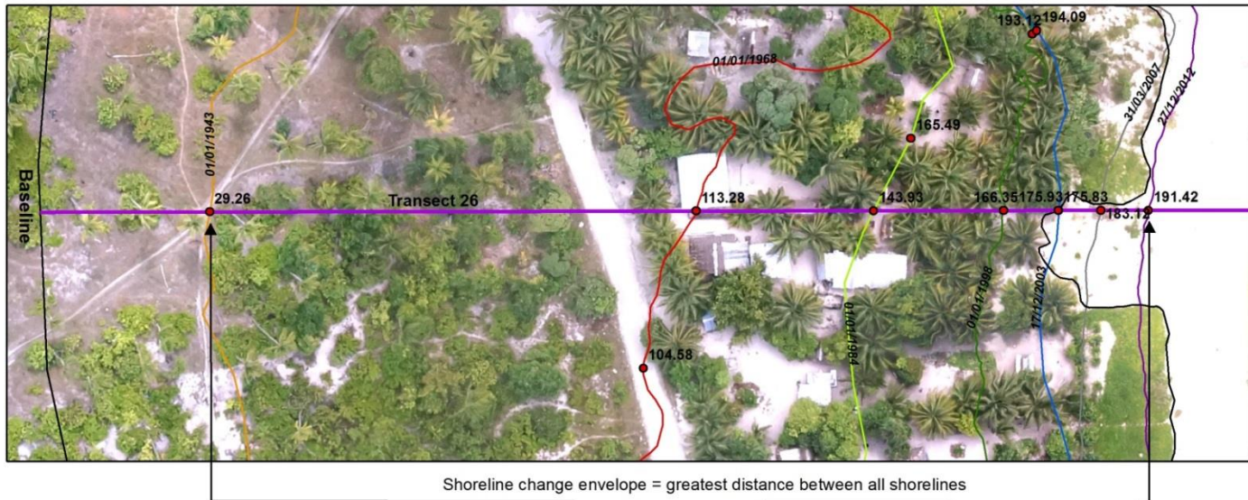
Figure 10: Shoreline change envelope for Transect 26, which was on the ocean side of Bonriki
