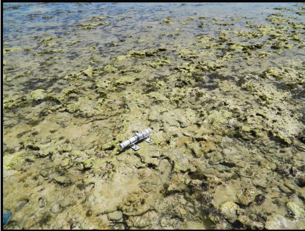
Figure 7: Tide and wave recorder deployed on the reef flat east of Bonriki.
