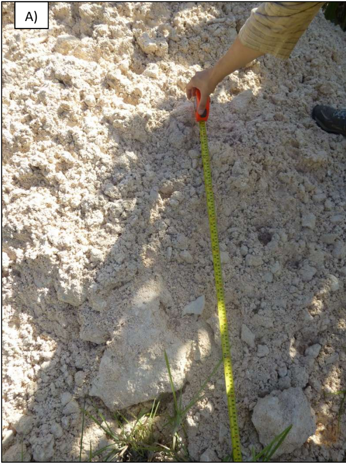
Figure A5.4: Rock samples at piezometer – BN1B, Bonriki (14/11/13). A) Gravelly sand + coral boulders (depth 2.20 - 2.40m); B) Coral boulder.
