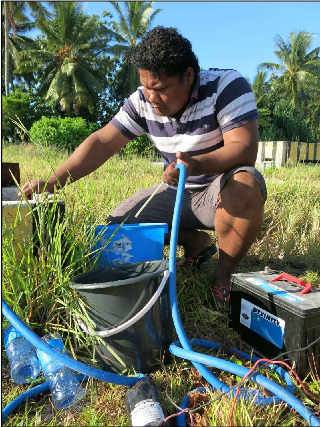
Figure 12: Sampling equipment used by MPWU staff members in the field, 12-V diaphragm pump (foreground), used to abstract water from 8-mm sampling tubes that can then be measured for salinities or other purposes.
