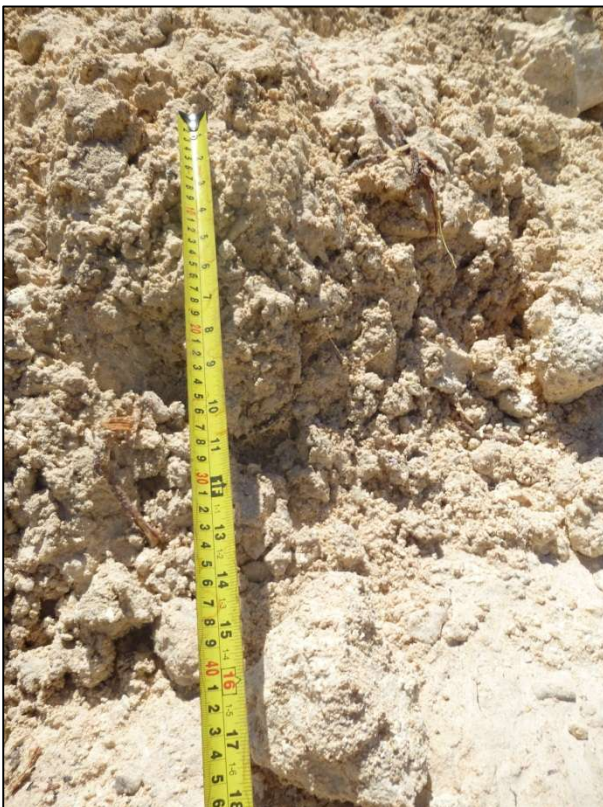
Figure A5.17: Rock samples at piezometer – BN20B, Bonriki (16/11/13).Sandy gravel.
