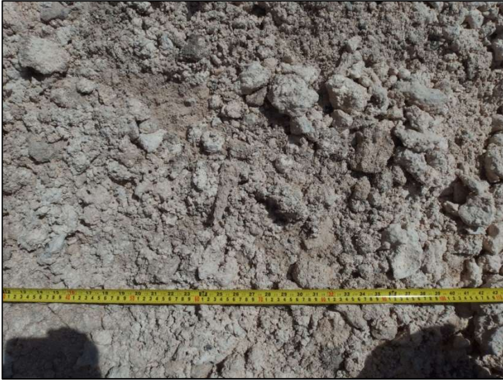
Figure A5.15: Rock samples at piezometer – BN15B, Bonriki (14/11/13). Sandy gravel.
