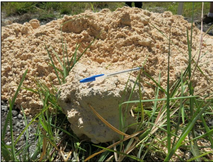
Figure A5.19: Rock samples at piezometer – BN23B, Bonriki (14/11/13). Silty sand, fine to medium, with gravel and coral boulders.
