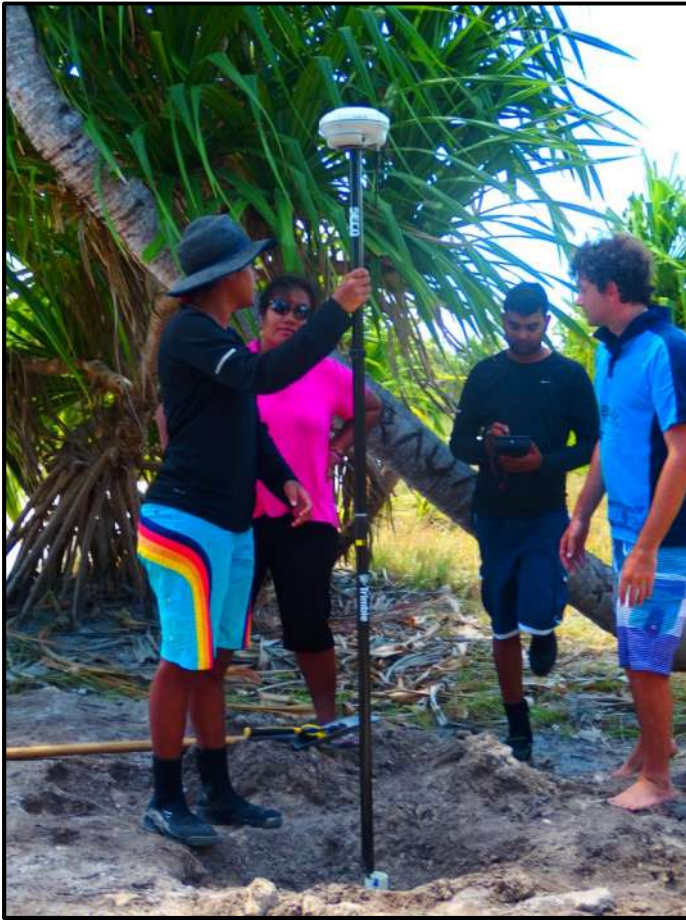
Figure 16: Using an RTK rover unit to measure the elevation to the Top of Pipe measuring point in piezometer BN35.
