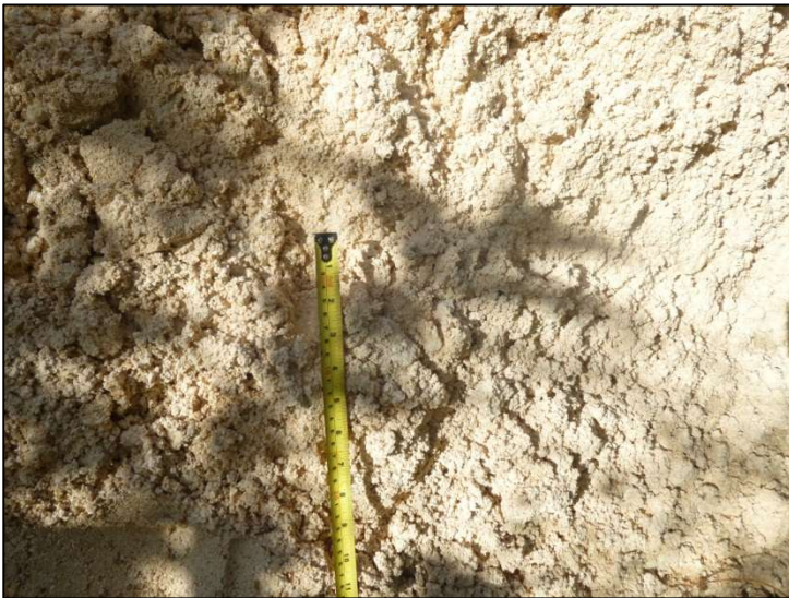
Figure A5.21: Rock samples at piezometer – BN35, Bonriki (16/11/13). Gravelly sand.
