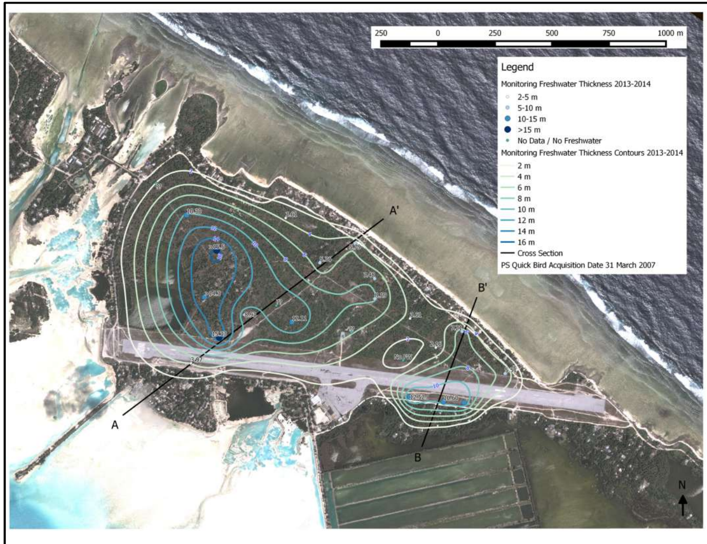
Figure 32: Contour map of the freshwater lens thickness from monitoring boreholes averaged over 2013–2014, with cross section profiles A–A' and B–B'.
