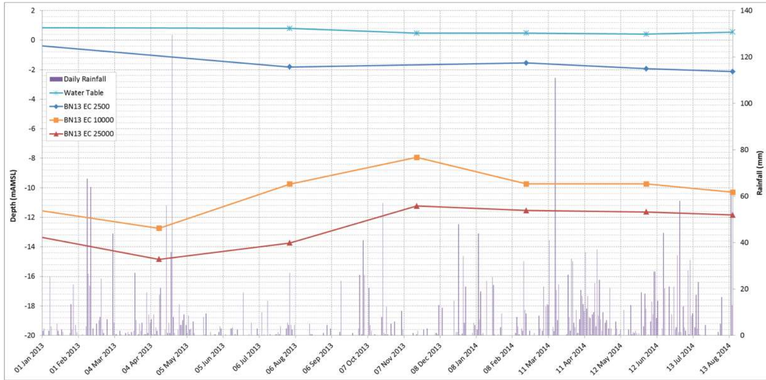
Figure A12.11: Recent salinity variations at monitoring location BN13.
