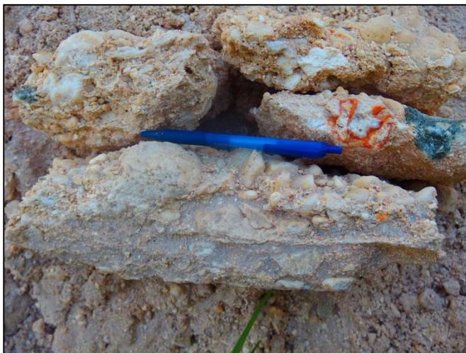
Figure A5.9: Rock samples at piezometer – BN7B, Bonriki (15/11/13). Beach rock (conglomerate formation).
