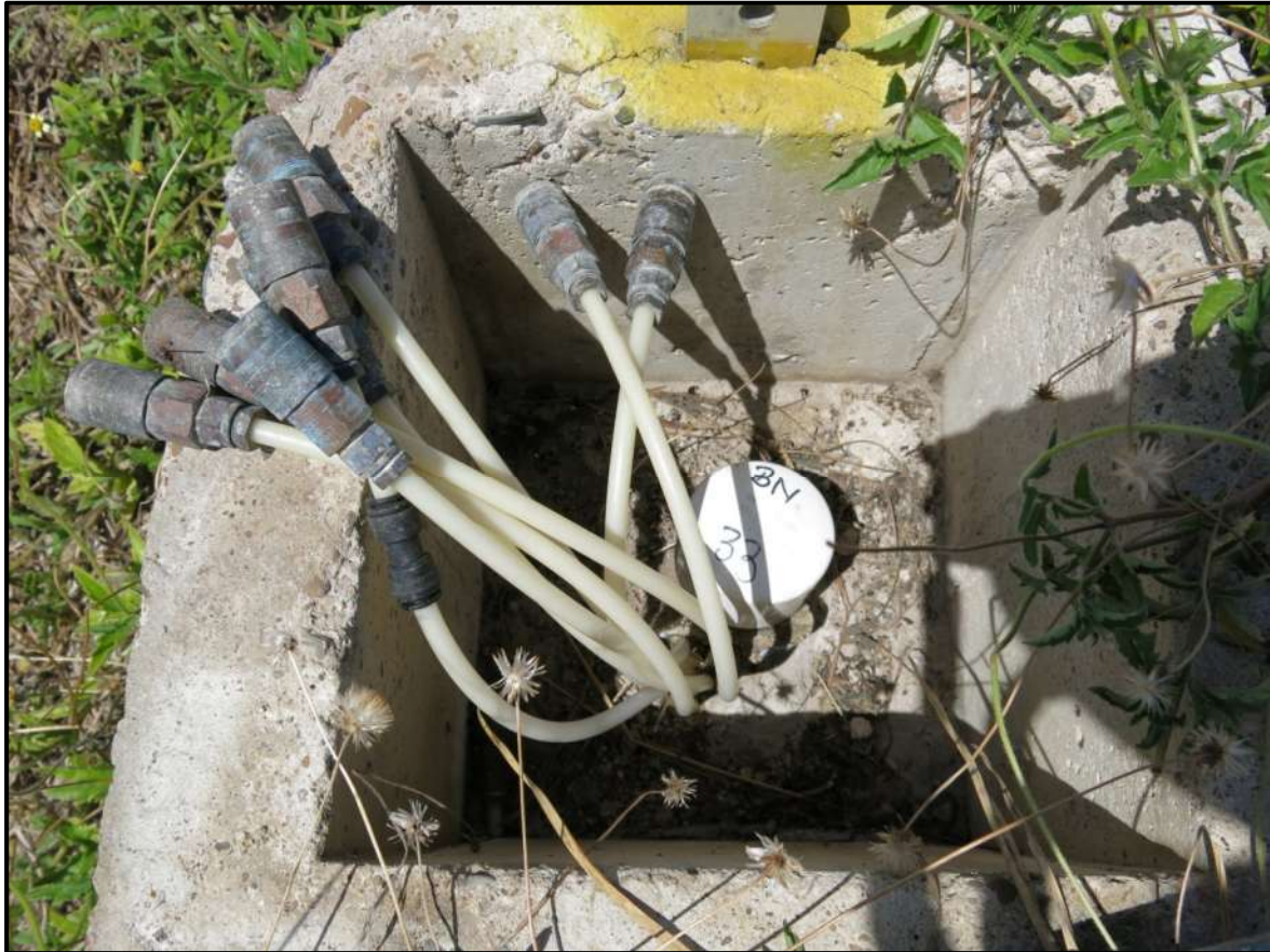
Figure 11: Seven sampling tubes at selected depths with RYCO fittings, and 50-mm PVC piezometer to the water table within BN33 monitoring borehole box.
