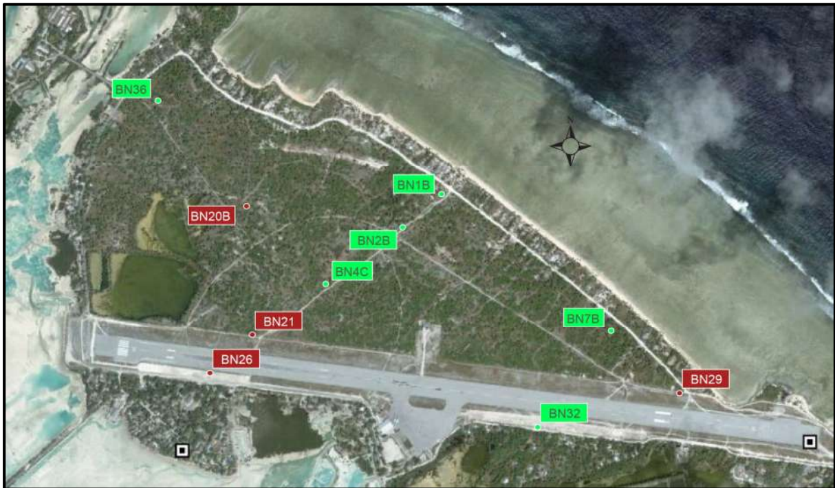
Figure 28: Location of the 10 conductivity, temperature, and depth divers (divers installed November 2013 to March 2014, green colour, and divers installed November 2013 to June 2014 red colour). The barometric diver was located at monitoring borehole BN26.
