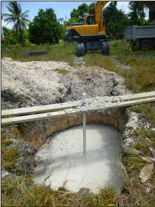
Figure A5.16: Lithology log at piezometer – BN20B, Bonriki (16/11/13).
