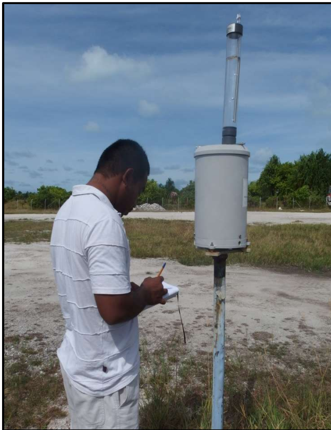
Figure 5: Calibrating the Bonriki airport TB3 rain gauge station.
