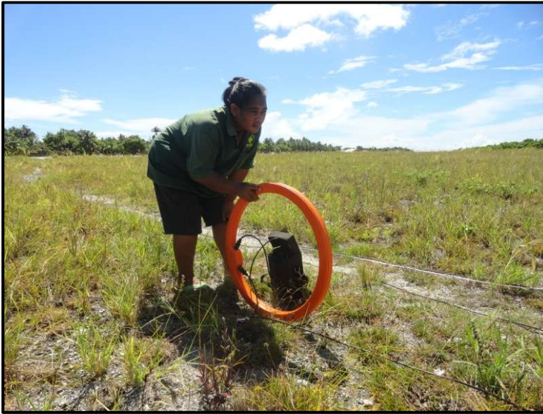
Figure 18: Ministry of Public Works and Utilities staff member undertaking EM34 surveys.
