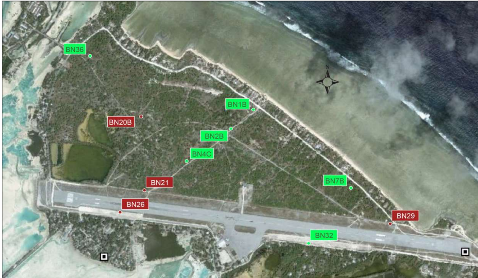
Figure A10.1: Location of the 10 CTD divers (divers denoted in green installed Nov 2013–March 2014; divers denoted in red installed Nov 2013–June 2014). The barometer diver was located in BN26.
