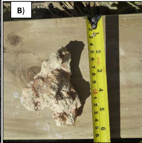
Figure A5.4: Rock samples at piezometer – BN1B, Bonriki (14/11/13). A) Gravelly sand + coral boulders (depth 2.20 - 2.40m); B) Coral boulder.
