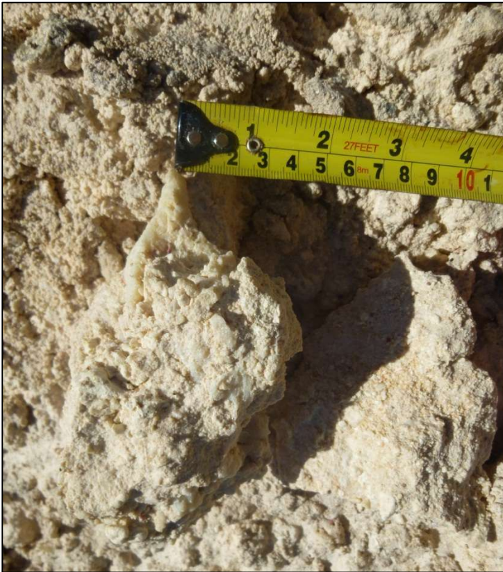
Figure A5.23: Rock samples at piezometer – BN36, Bonriki (16/11/13). Gravelly sand with sandstone boulders.
