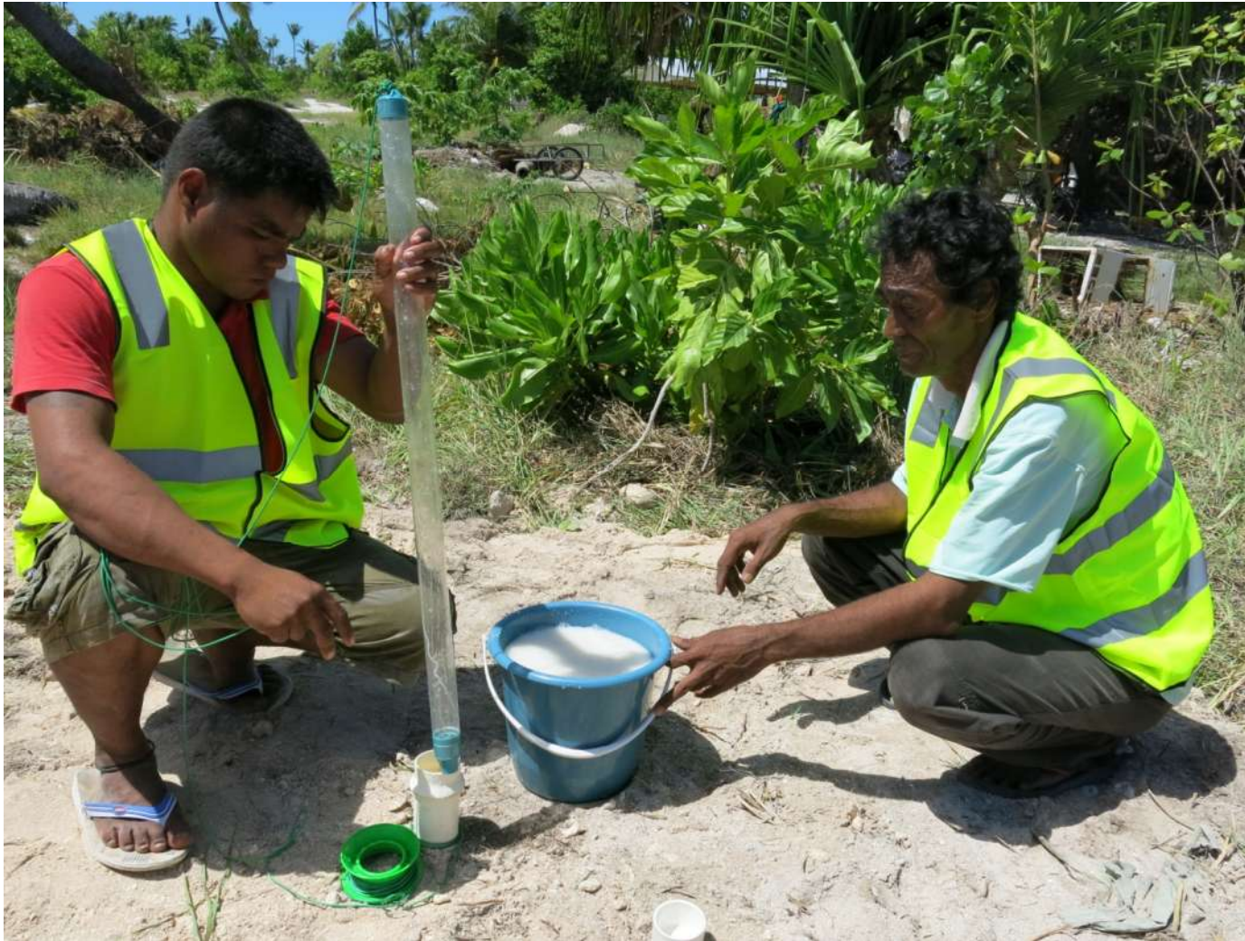
Figure A5.29: Bailing of piezometer to clear silt and develop well until clear sample is obtained – BN1.
