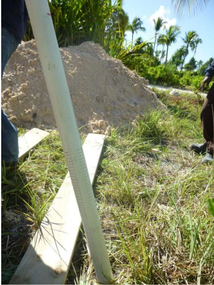
Figure A5.25: Machine-cut PVC screen.
