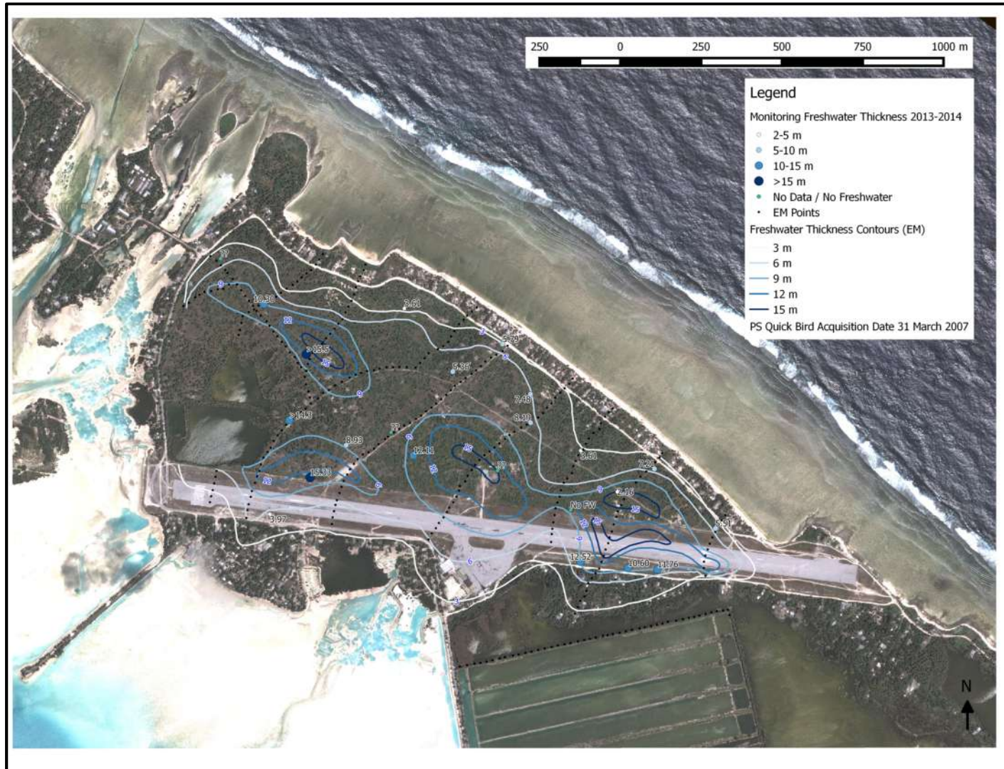
Figure 33: Contour map of freshwater lens thickness from EM34.
